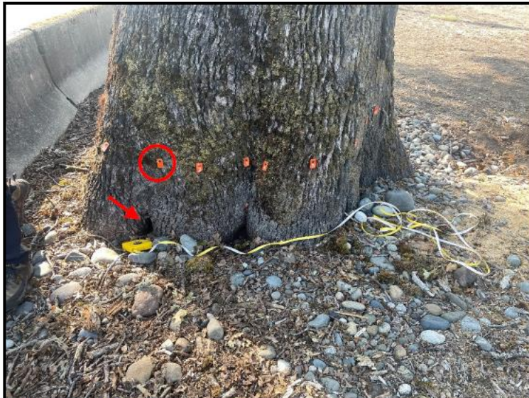
Photograph 1. Measuring point 1 is circled in red. An opening into the decay cavity is indicated by the red arrow.
